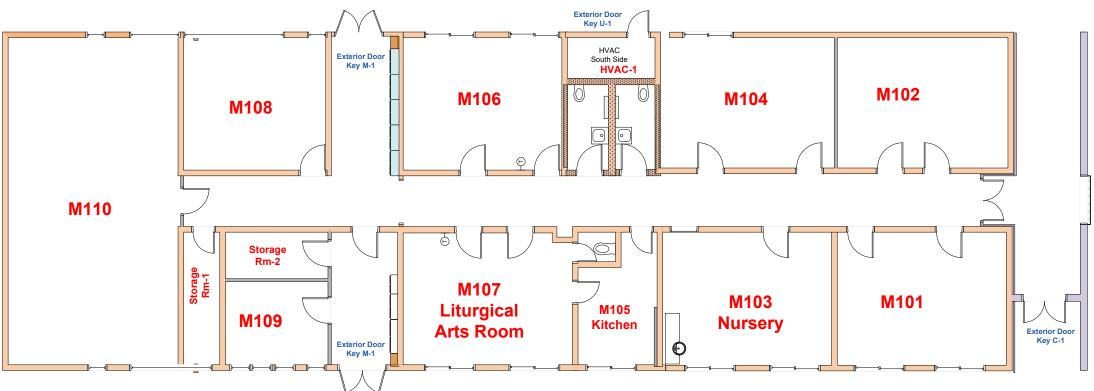
Mission Wing has two heating systems. One controls the South side of building the other the North side. South side thermostat is located in Room M106 North side thermostate is located in Room M107
